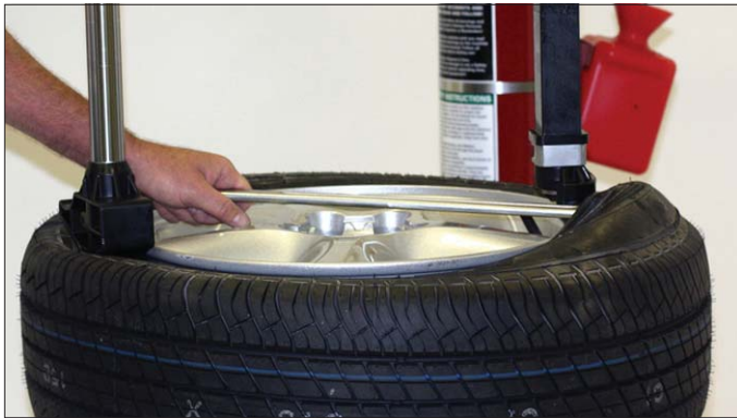
Figure 13 - Lift Bead Over Demount Tool
