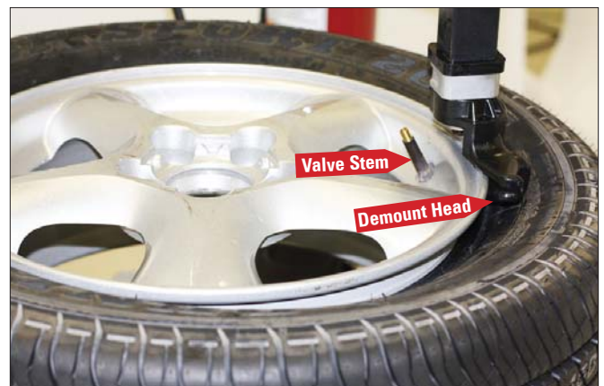
Figure 36 - Position Valve Stem Under Demount Tool
