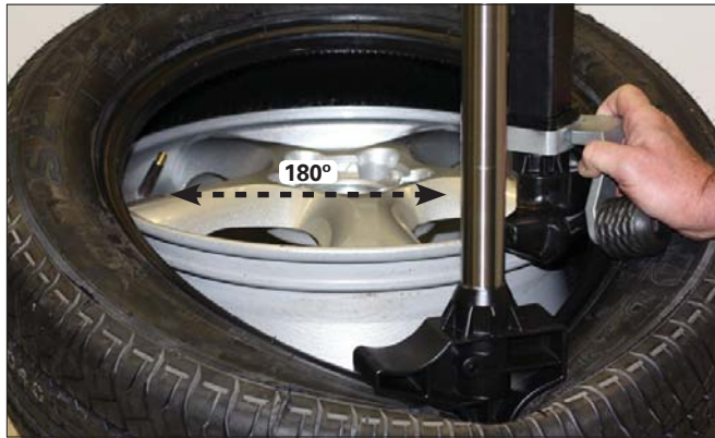
Figure 43 - Position Valve Stem 180° Ahead of Mount/Demount Tool
