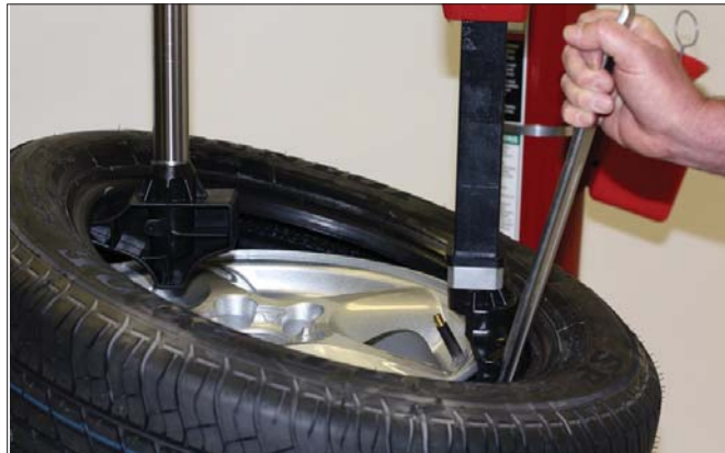
Figure 41 - Rotate Lifting Tool Down for Demount
