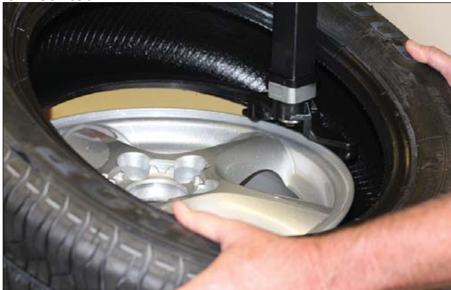
Figure 20 - Mounting Lower Bead
