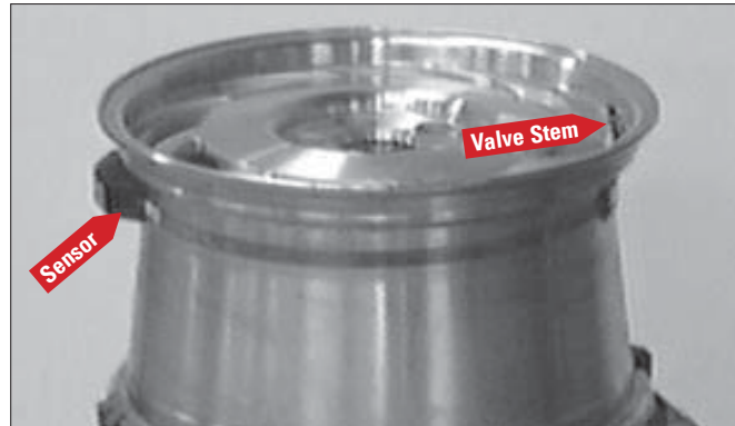
Figure 31 - Wheel with Low Pressure Sensor/Transmitter
