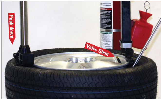
Figure 12 - Insert Bead Lifting Tool
