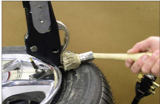
Figure 49 - Apply Lubricant to Bead Lifter Tool Hook
