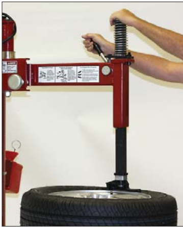
Figure 8 - Position Mount/Demount Tool
