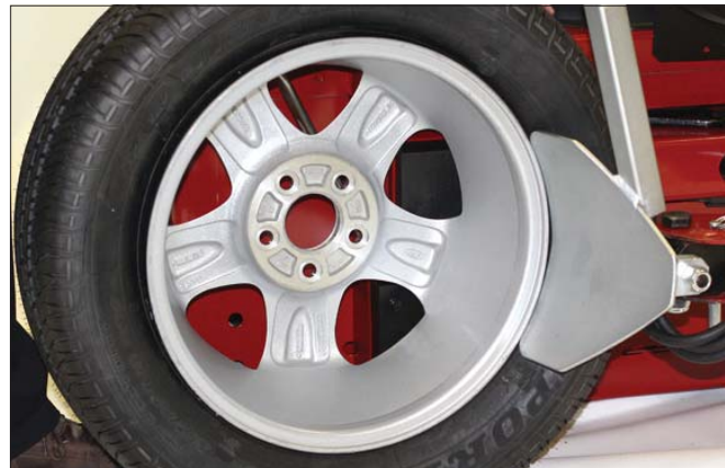
Figure 32 - Loosen Bottom Bead
