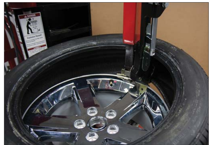
Figure 55 - Demount Lower Tire Bead
