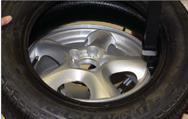
Figure 19 - Position Tire Against Mount/Demount Tool
