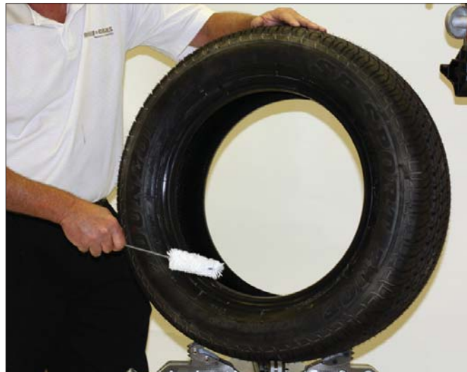
Figure 18 - Lubricate Tire Beads Liberally
