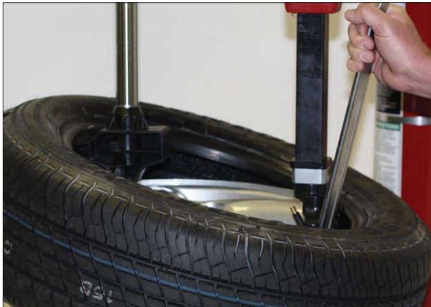
Figure 14 - Demounting Lower Bead
