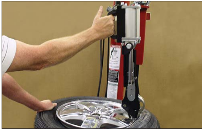
Figure 51 - Leverless Tool Hooked Under Tire Bead
