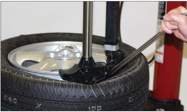
Figure 37 - Insert Bead Lifting Tool
