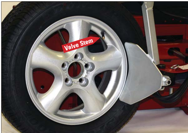
Figure 29 - Position Tire for Bead Loosening
