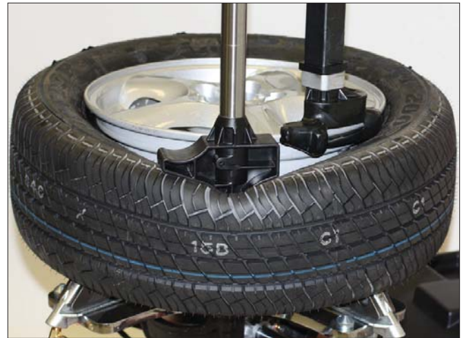
Figure 34 - Helper Foot Depressing Sidewall of Tire
