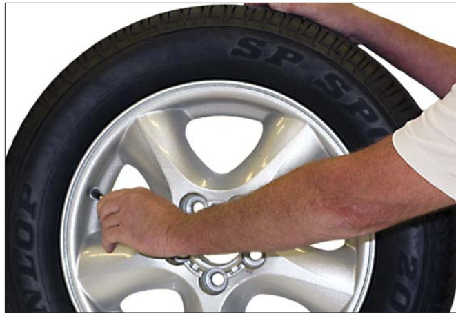
Figure 1 - Remove Valve Core to Deflate Tire
