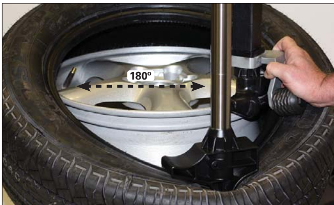
Figure 21 - Position Valve Stem 180° Ahead of Mount Tool
