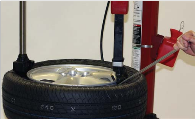
Figure 38 - Helper Foot Pushing Bead Into Drop Center
