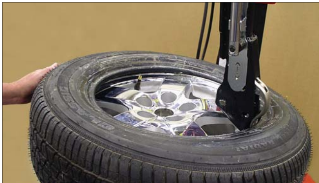
Figure 52 - Demount Upper Tire Bead
