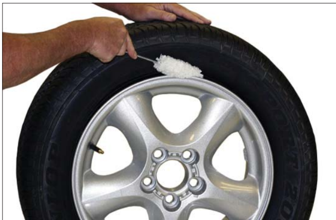
Figure 5 - Apply Rubber Lubricant to Tire Beads
