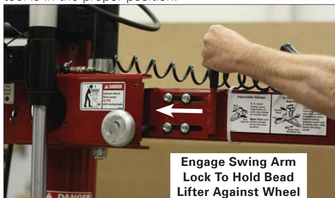
Figure 48 - Lock Swing Arm In Position
