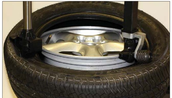
Figure 24 - Mounting Top Bead
