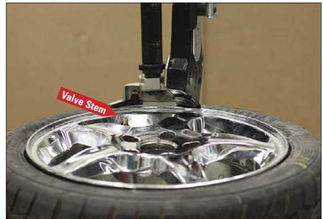
Figure 50 - Position Valve Stem Behind Leverless Demount Tool
