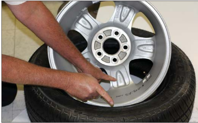
Figure 16 - Verify Size Match Between Tire and Wheel
