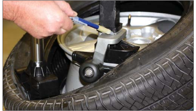
Figure 22 - Duckhead Roller Properly Mounted On Bracket
