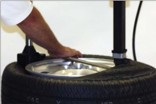
Figure 39 - Rotate Lifting Tool Down for Demount
