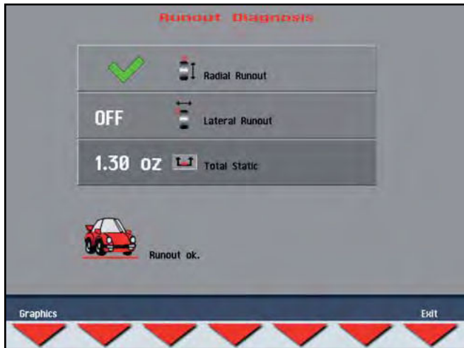
Figure 25 - Runout Diagnosis Screen
