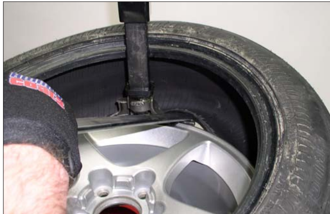
Figure 13- Guide Bead Over Tool Head
