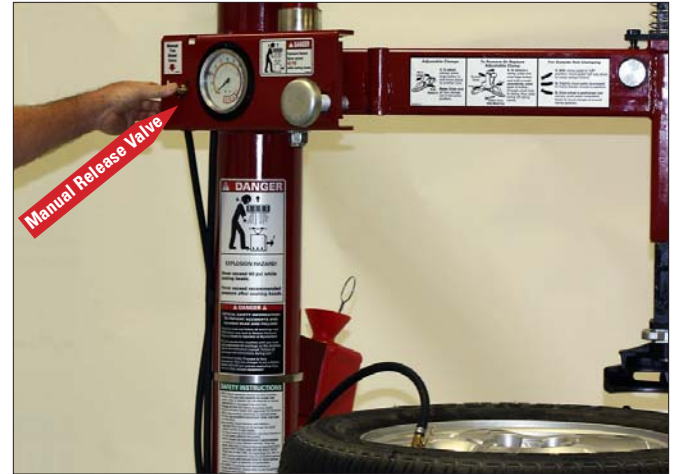
Figure 27 - Location of Manual Release Valve
