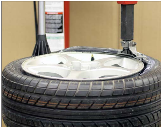
Figure 24 - Use Bottom of Robo-Arm LR Foot to Flip Bead Over Rim Flange
