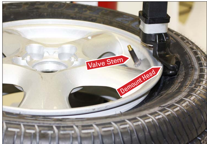
Figure 17 - Position Valve Stem Behind Demount Tool Tail
